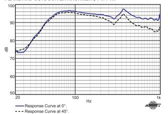
Response curves measured on ground plane and outdoor environment with the subwoofer installed in a test enclosure, 1 W / 1 m. This curves was decreased 6 dB to compensate the ground plane gain.
